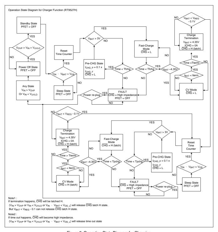
Figure 3. Operation State Diagram for Charging
