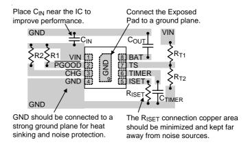
Figure 2. PCB Layout Guide
