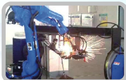
Mechanical hand welding
