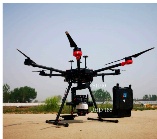
Figure 3. Unmanned aerial vehicle (UAV) hyperspectral imaging system.
