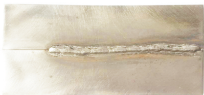
Butt welding effect of 0.5mm plate
