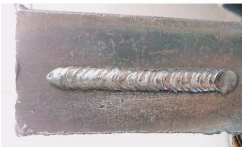
cellulose electrode vertical down welding effect
