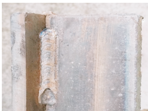
cellulose electrode vertical down fillet welding effect
