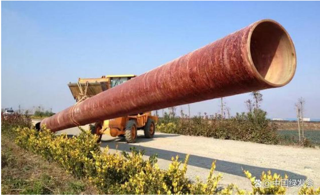
The center and a Zhejiang company successfully developed the bamboo composite pipe
