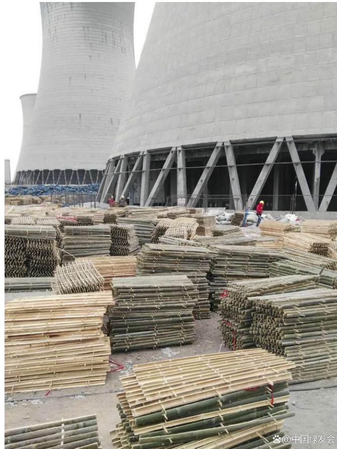
The center and a company in Jiangsu successfully developed bamboo material for power plant cooling tower
