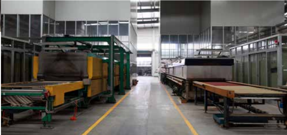
The continuous flat tempered glass production furnace (W:1500 x L:5000mm) 连续式平钢化窑炉 (宽:1500 x 长:5000 mm)
