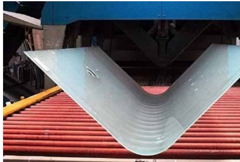
The continuous flat tempered glass production furnace (W:1500 x L:5000mm) 连续式平钢化窑炉 (宽:1500 x 长:5000 mm)
