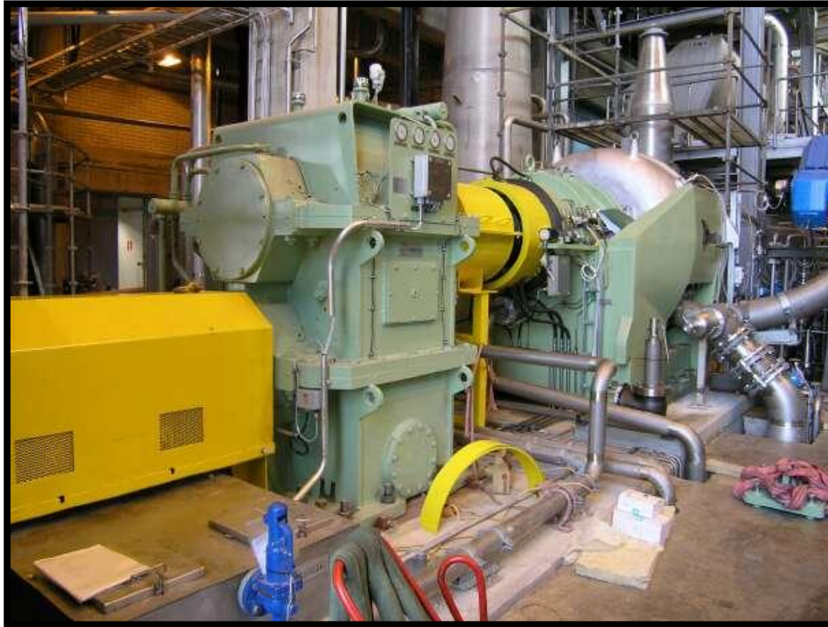
Single stage gear unit (increaser) 32 MW motor power
