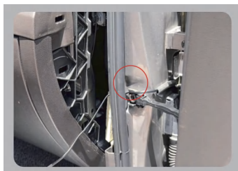
② Thread the camera video cable into the car from below the door seal
