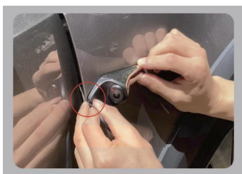
① Fix the camera at the edge of the car door
