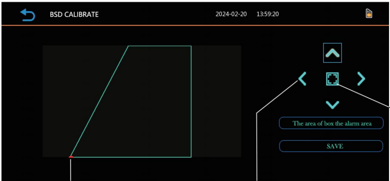
Calibrate the warning range by moving the set point
