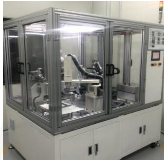
砷化镓太阳能电池半自动贴玻璃盖片设备 Solar cell automatic glass cover equip
