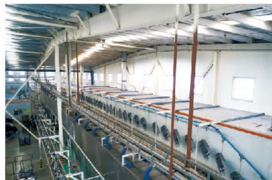
全封闭喷淋式前处理流水线 Large fully enclosed spray pre treatment assembly line
