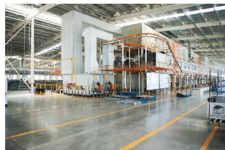
大型全封闭无尘自动喷涂线 Large-scale fully-enclosed dust-free auto matic powder coating line
