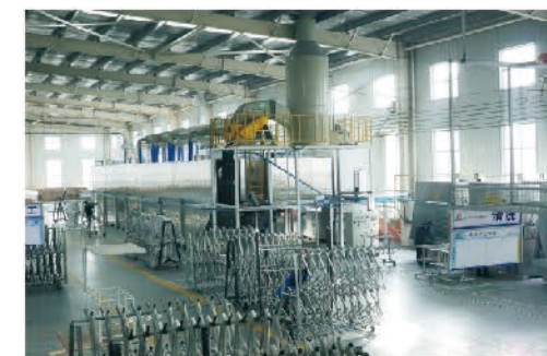
铝制品T4固溶和T6时效炉T4 & T6 Heat treatment T4&T6
