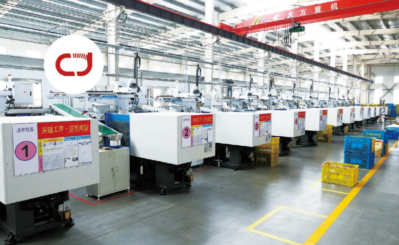
全自动注塑线和转盘式发泡生产线 Automatic injection molding process, plastic production line and PVC foaming line
