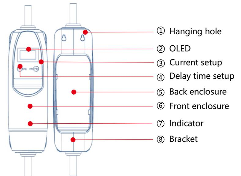
Figure 2 Front and Back of the EV Charger
