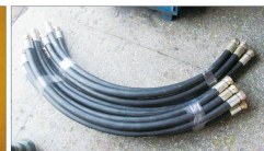
Hydraulic oil pipes
