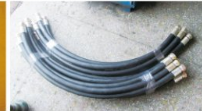
Hydraulic oil pipes
