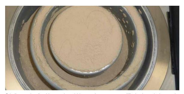
Grinding results after 20 seconds and 30 seconds appear not to differ by the optical properties. Both times, sample was sticking lightly to core and ring (easy to brush off). Only by sieving, it was shown that the 30 seconds grinding result is finer.
