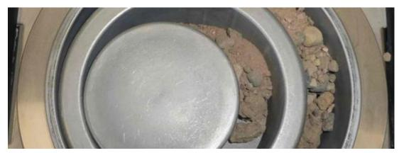
Sample and gravel and sand got pre mixed with a small shovel. Afterwards, 100 grams have been filled into the grinding set. About 1/3 of sample was placed between core and ring.
