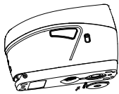
Fasten the buckle on the replacement measuring aperture
