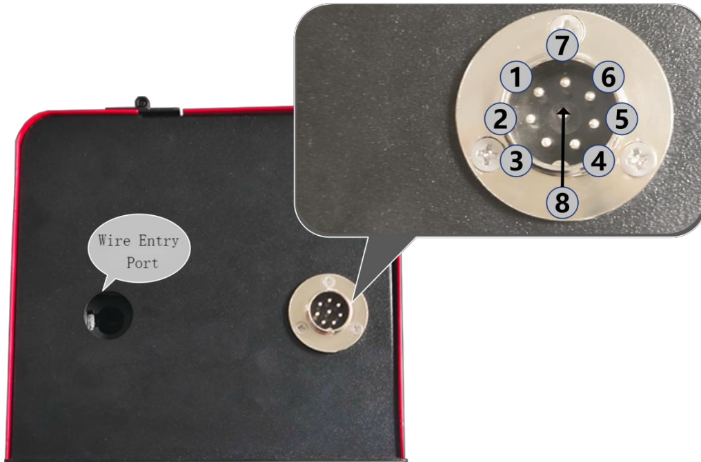
Figure 4.1 Diagram of the aviation plug-in interface
