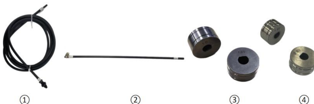
Fig. 4.3 Schematic diagram of wire feeding tube and wire feeding wheel
