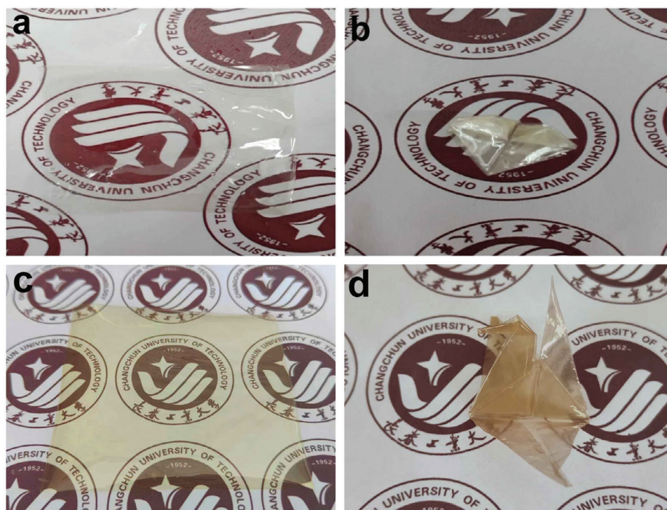
Figure 4. The transparency and flexibility of membranes. a,b): SP-2MIMO 132-5 ; c,d): SP-Mo 72 Fe 30-3 .
