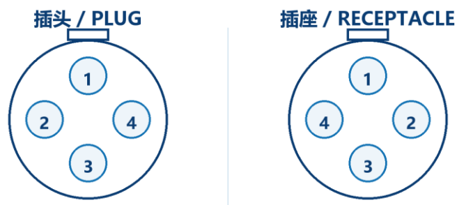
SHS-4光插合面视图 / SHS-4 MATING-FACE VIEW
