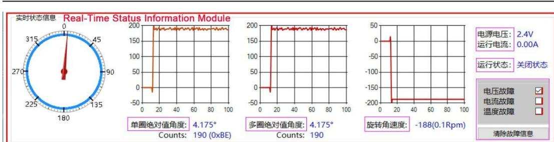
This functional module displays the current single-turn absolute angle, multi-turn absolute angle, speed, power voltage, operating current, operating status, fault information, etc. of the current motor in real time.
