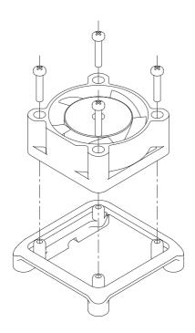
3. Remove four long screws and four nuts on the air unit.
