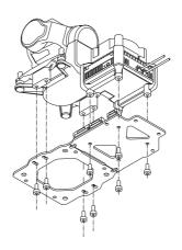
4. Fix the Antenna Mount on the Integrated Base Plate with two M2 x L6mm tapping screws, and snaps the antennas into the Antenna Mount.
