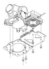
6. Fix the Antenna Mount on the Integrated Base Plate with two M2 x L6mm tapping screws, and snaps the antennas into the Antenna Mount. (Diagram refer to *Installing Gimbal and DJI O4 Pro – step 4* in this manual)
