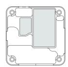
3. Install the housing with four M1.6 x L4mm machine screws.
