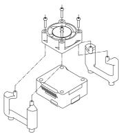
3. Fix the gimbal on the Integrated Base Plate with four M2 x L4mm machine screws. Connect the power-communication port of the gimbal and the gimbal transferring port with a Gimbal Transferring Cable.
