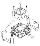
3. Fix the gimbal on the Integrated Base Plate with four M2 x L4mm machine screws. Connect the power-communication port of the gimbal and the gimbal transferring port with a Gimbal Transferring Cable.
