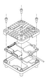
4. Fix the Cooling Fan on the air unit with four M2 x L12mm machine screws.
