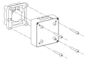
5. Fix the Moonlight Air Unit Mount on the air unit with four M2 x L4mm machine screws.
