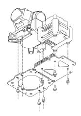
4. Fix the Antenna Mount on the Integrated Base Plate with two M2 x L6mm tapping screws, and snaps the antennas into the Antenna Mount. (Diagram refer to *Installing Gimbal and DJI O4 Pro – step 4* in this manual)
