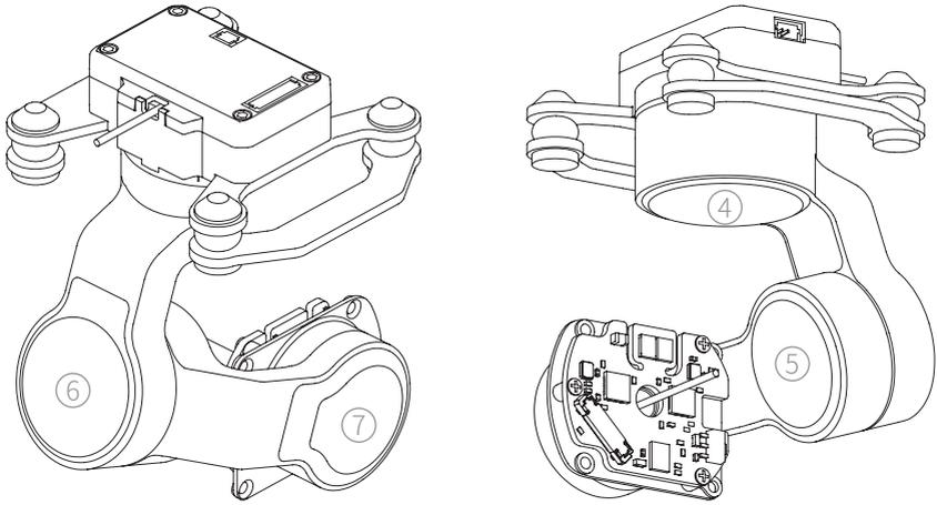
5. Mount the payload device onto the gimbal by four M1.6 countersunk head screws.
