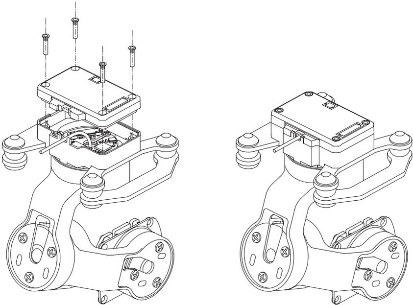
3. Route the payload cables through the roll motor and the pitch motor in sequence.
