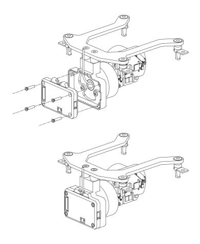
3. Route the payload cables through the pitch motor.
