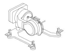
5. Mount the payload device onto the gimbal by four M1.6 countersunk head screws.
