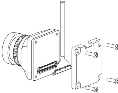
3. Insert the coaxial cable through the groove on the side of the gimbal.
