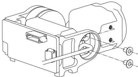
4. Connect the coaxial cable from the gimbal to the air unit and reinstall the cover back.
