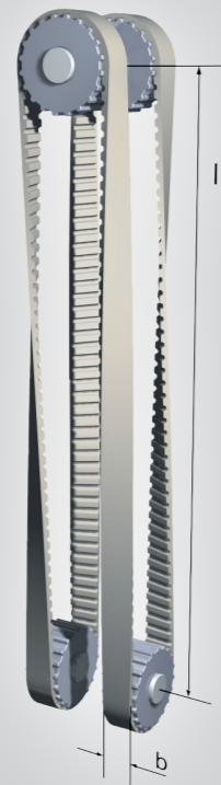
2 轴扭向传动装置 Angular drive with 2 axes
