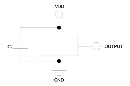
AMLX90248's pole-independent sensing technique allows for operation with either a north or south poles magnet orientation, enhancing the manufacturability of the device. The state-of-the-art technology provides the same output polarity for either pole face.
