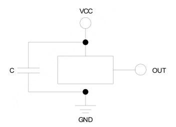
AMT6133's pole-independent sensing technique allows for operation with either a north or south poles magnet orientation, enhancing the manufacturability of the device. The state-of-the-art technology provides the same output polarity for either pole face.
