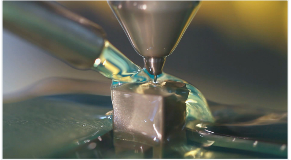
Sarix 3D EDM milling technology in action. KunLun has the Sarix machine in factory being utilized for creating micro mold inserts.
